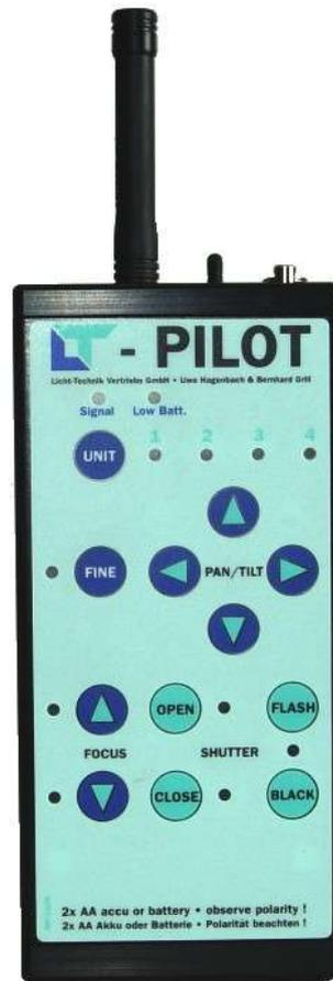
The **UNIT** – button selects the desired unit. One of the LEDs on the right side indicate the current unit.
