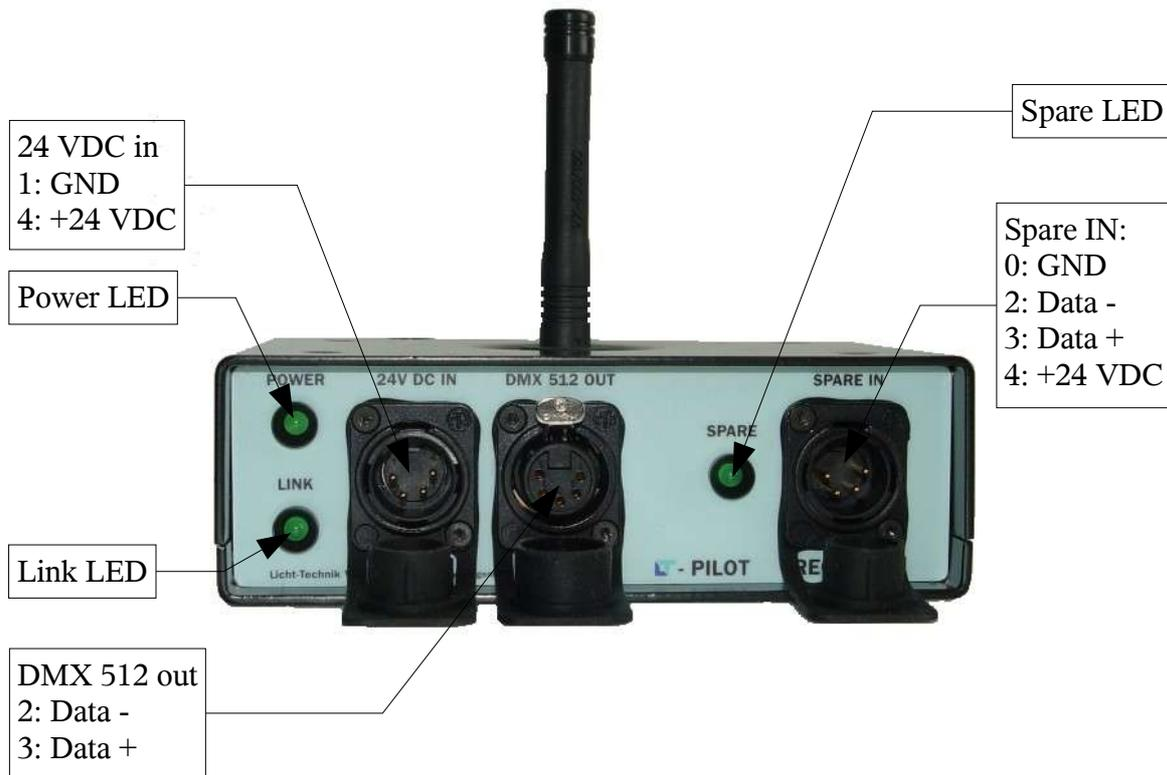
**Power LED:** Is on, if there is power on the 24V DC in input.
