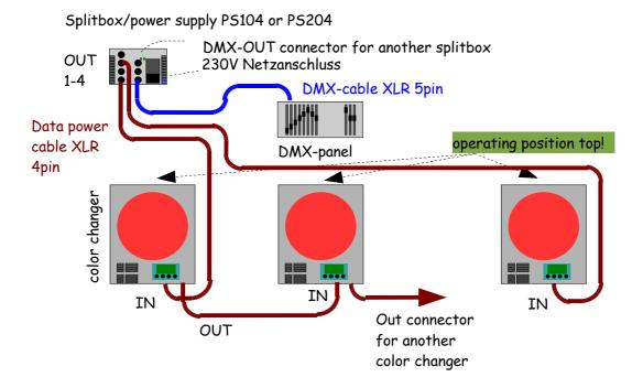
Connect the light mixer panel and the Splitbox PS104/PS204 with a 5PIN XLR-DMX-cable. The splitbox is provided with a DMX out jack for connecting additional splitboxes. At each of the four DATA Power outputs for the devices a maximum of 4 color changers can be connected. However, the total number of Color Changers per splitbox must not exceed 16 color changer (PS204) or 8 Color Changer (PS104) respectively.
