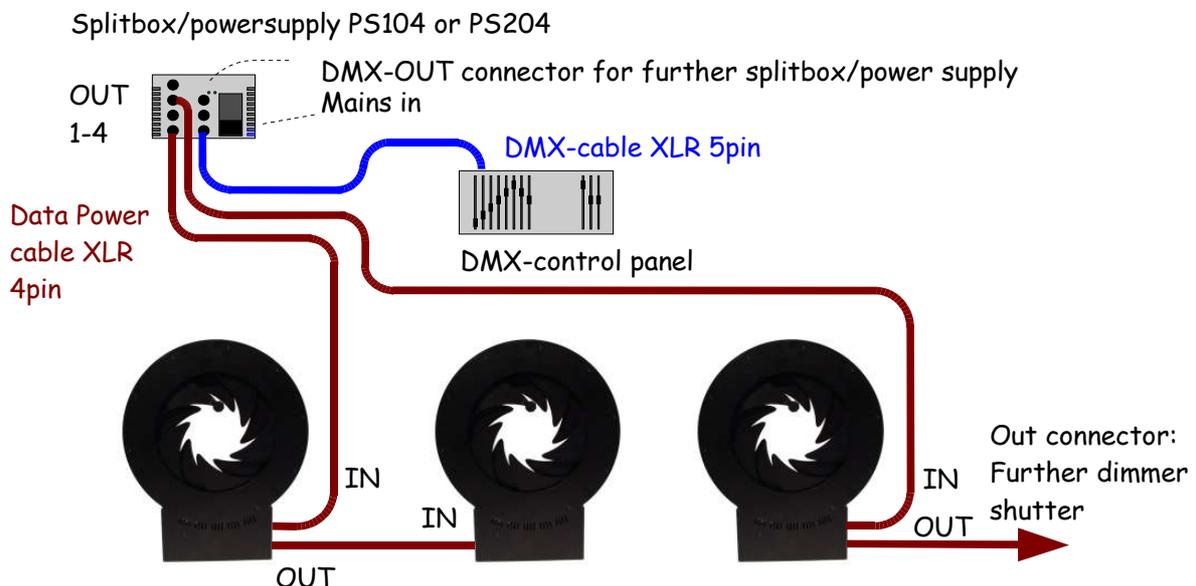
Connect the light mixer panel and the splitbox PS104/PS204 with a 5PIN XLR-DMX-cable. The splitbox is provided with a DMX out jack for connecting additional splitboxes. At each of the four DATA Power outputs for the devices a maximum of 8 BladeFaders can be connected. However, the total number of MagVaders per splitbox must not exceed 26 devices (PS204) or 13 devices (PS104) respectively.
