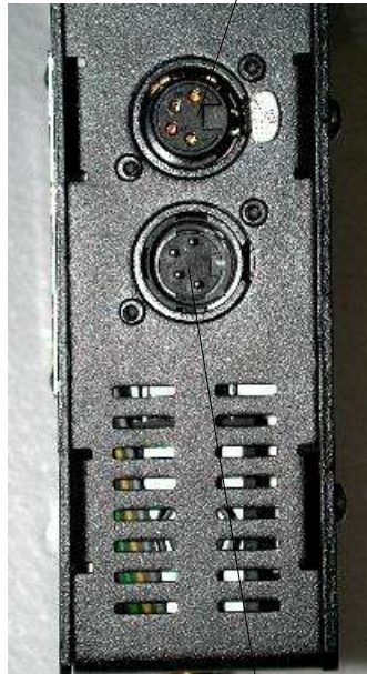
4pin output possibility for another Bag o Light system OR Inflator fan connector
