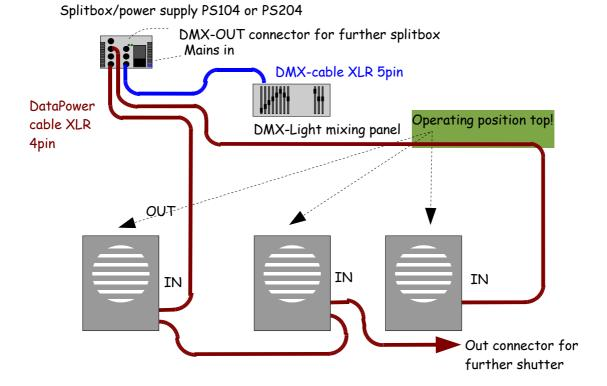
Connect the light mixer panel and the Splitbox PS104/PS204 with a 5PIN XLR-DMX-cable. The splitbox is provided with a DMX out jack for connecting additional splitboxes. At each of the four DATA Power outputs for the devices a maximum of 8 Shutters can be connected. However, the total number of Shutters per splitbox must not exceed 16 (PS204) or 8 (PS104) respectively.
