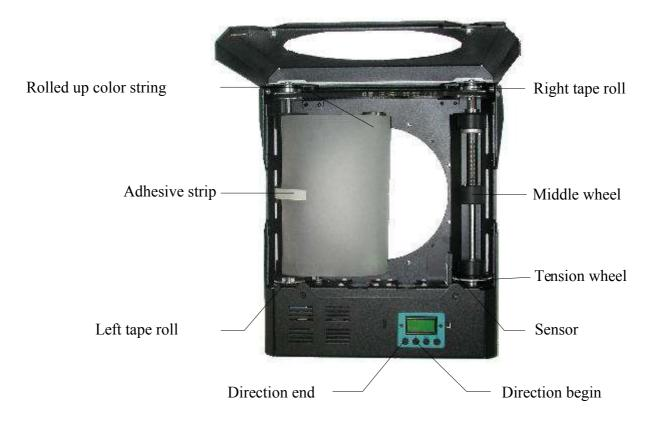
Roll up the tape so that the tail leader is the open end. Put in the color string like on the picture above and fix the tape with a high temperature adhesive strip on the middle wheel of the left roll. Now you can roll up the tape comfortably with the color changer using the key DOWN (direction begin). The UP button moves the tape in the other direction.
