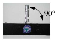
Furthermore, the **spigot** itself and the **surface** of the yoke must not be deformed. Make sure that the spigot is not loose.
