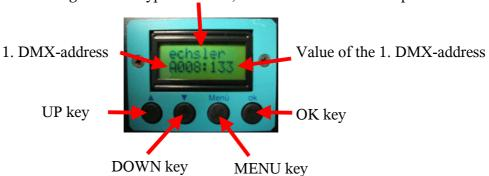
In normal operating mode the **LCD-display** indicates different information. The first line shows the Licht-Technik moving text with details on type of device, software version and telephone number. The second line indicates the first DMX-address and its incoming value (8-Bit, 0..255). For the motoryoke, this address is the PAN-address.
