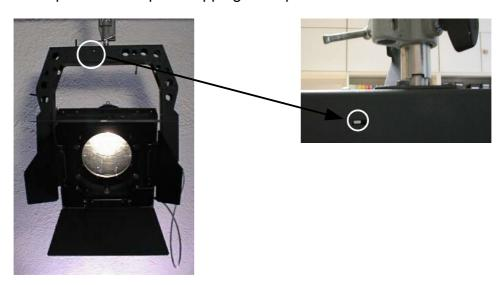
**For understanding:** Because of exerting the tripping lever, the motoryoke remains **internally** on its middle position. The absolute value device does not join in turning anymore. You turn the yoke around this internal middle position.
