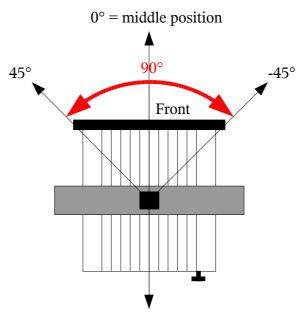
This setup is useful when the motoryoke is hanging in a **corner** for example. Setting the PAN middle position:
