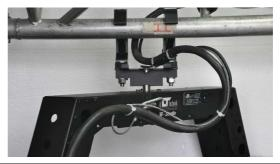
Wrong routed cables can lead to defective cables, because of the mechanical and thermic influence!
