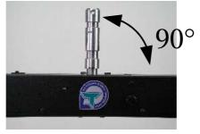
Furthermore, the **spigot** itself and the **surface** of the yoke must not be deformed. Make sure that the spigot is not loose or unformal.
