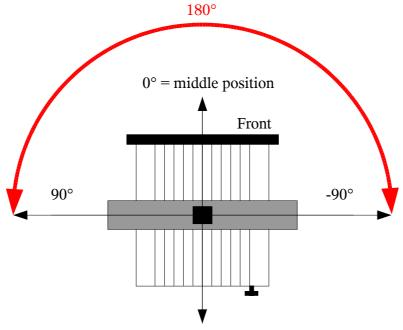
If an angle of 45° is programmed, the yoke will move 45° to the left and right. The moving range is 90°.
