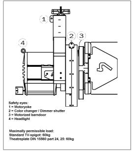
Make sure that the safety belts have the right diameter. For weights up to 60 kg a belt of 10mm diameter is necessary for the one way method and a belt of 6mm is necessary for
