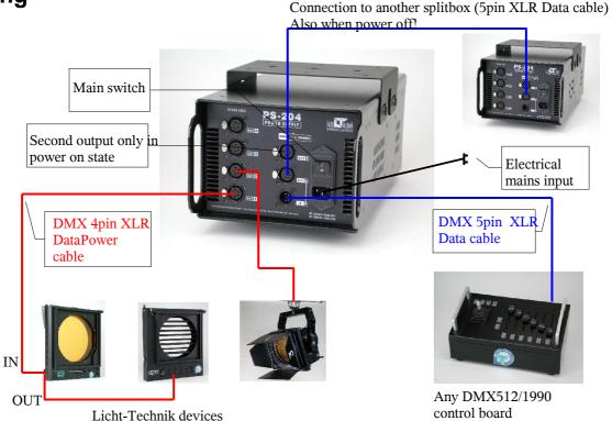
The standardized DMX-Signal is based on industrie's RS485 Interface. It is designed for maximum lengths up to 1200m. This length is under condition in theatre or studio normally not possible. As a result of internal tests we recommend a maximum length of 200m (only DMX, 5PIN). A maximum of 32 DMX receiver can be connected to one DMX transmitter. If more devices should be connected a splitbox must be used.
