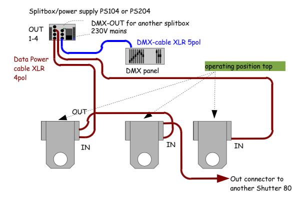
Connect the light mixer panel and the Splitbox PS104/PS204 with a 5PIN XLR-DMXcable. The splitbox is provided with a DMX out jack for connecting additional splitboxes. At each of the four DATA Power outputs for the devices a maximum of 8 Shutters can be connected. However, the total number of Shutters per splitbox must not exceed 16 (PS204) or 8 (PS104) respectively.
