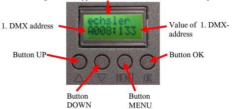
The **LCD-Display** indicates several information in normal operation mode. The first line shows a moving text with service telephone number. The second line shows the current DMX address and the incoming value (0..255).
