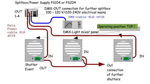
Connect the light mixer panel and the Splitbox PS104/PS204 with a 5PIN XLR-DMX-cable. Splitbox is provided with a DMX out jack for connecting additional splitboxes. At each of the four DATA Power outputs for the shutters a maximum of **8** shutters can be connected. The total number of shutters per splitbox must not exceed **32** Shutter Event (PS204) or **16** Shutter Event (PS104) respectively. Share the devices, so that every output is connected to the same number of devices.
