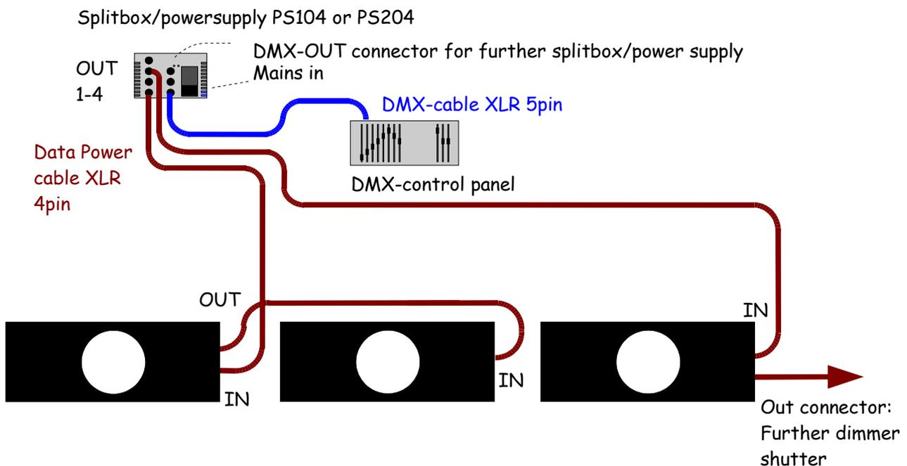
Connect the light mixer panel and the splitbox PS104/PS204 with a 5PIN XLR-DMX-cable. The splitbox is provided with a DMX out jack for connecting additional splitboxes. At each of the four DATA Power outputs for the devices a maximum of 8 Blackbeams can be connected. However, the total number of shutters per splitbox must not exceed 16 devices (PS204) or 8 devices (PS104) respectively.
